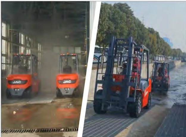
Automotive-grade rain shower, water immersion verification, imported connectors for excellent waterproof performance. IP65 protection level for lithium battery, safe and reliable.
