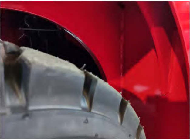
Adding rear wheel anti-splash mudguards for a cleaner battery compartment.
