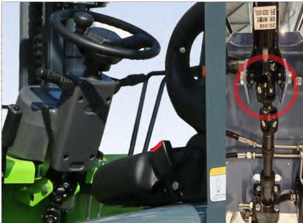
The new steering tube column locking mechanism which can adjust with less effort .
