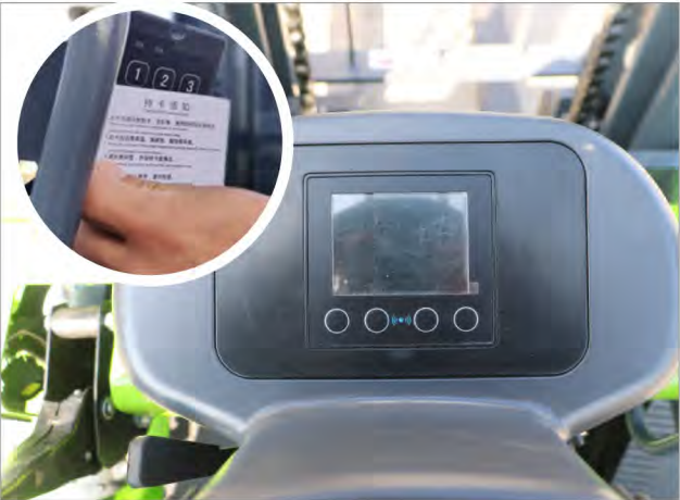
Swipe card activation, OPS down lock; The vehicle will automatically enter into sleep mode after 30 minutes of inactivity, making it safer and more energy-efficient.
